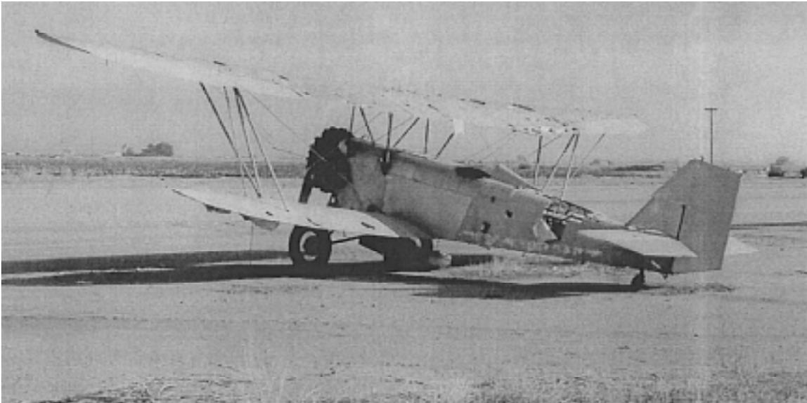
Above, an old New Standard D-25, registration and serial number unknown at Fram Field, Phoenix, Arizona. Could be NR31K, serial number 150 manufactured 1930. Note wire spoked wheels and condition of cotton fabric – completely rotted. Owner has obviously abandoned this aircraft because of its age and condition. Photo from Carl Small
