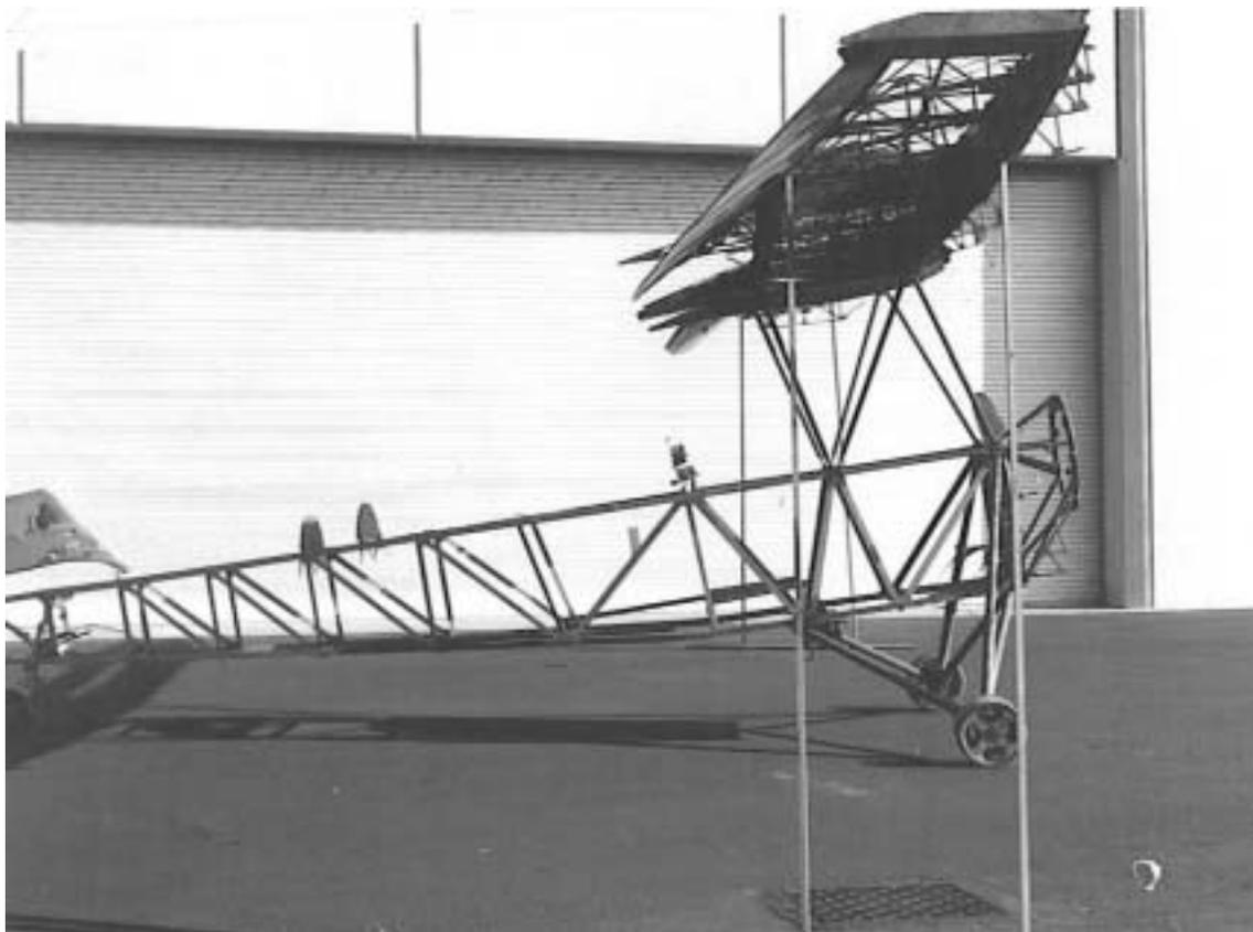
Above, New Standard D-25, NR9756 as assembled for first time after purchase. There was an engine, although it was totally disassembled and in boxes, a set of 30 x 5 wheels and a propeller. Think about deciding how to begin restoration! Photo from Budd Brockett, Reedley Exponent newspaper, Reedley, California
