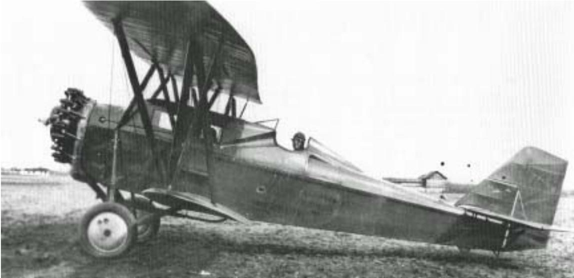
A rather different New Standard D-25, NC174H with factory-made canopy installed over the front cockpit. This created a cabin for the four passengers in the front, protecting them from weather and wind. Specially created for Alaskan Airways, Fairbanks, Alaska.
