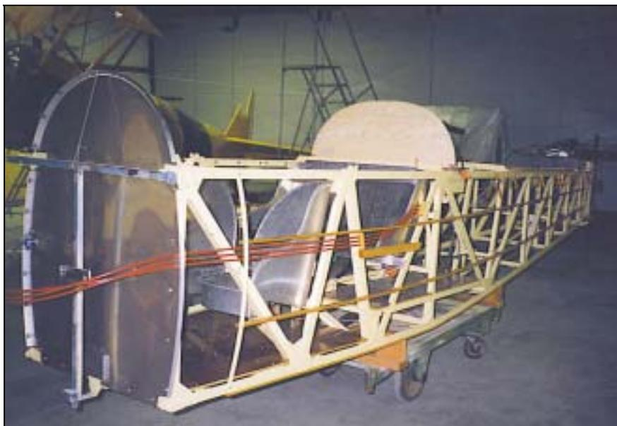
The fuselage frame with much of interior installed. Note all aluminum structure has been primed and painted to resist the effects of corrosion, a constant enemy of aluminum, particularly if the aircraft operates around a saltwater environment. The red lines are engine controls from rear throttle. Lockfoto
