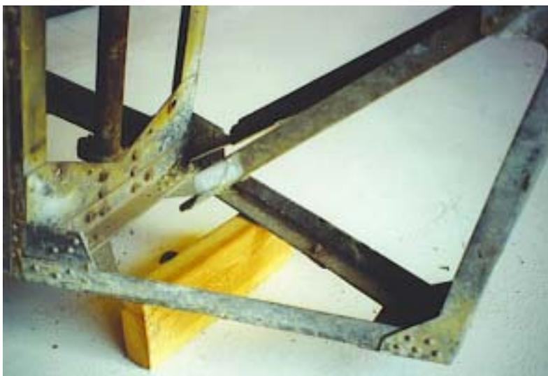
Left, corrosion has eaten away much of the aft fuselage of NR9756, necessitating replacement of much of the fuselage structure. Note that the diagonal aluminum angles are completely disintegrated by the effects of corrosion. Lockfoto
