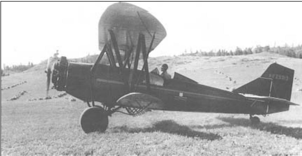
The very last New Standard manufactured was serial number 167W (W for White), NR25313. Note large rudder and extended vertical fin. Power is a Wright J-6-7 producing 285 hp and engine is equipped with a two-position Hamilton Standard propeller. Aircraft is possibly flown by Kenneth Tiegs who sprayed in the high country of Colorado. Photo from David B. Stevenson
