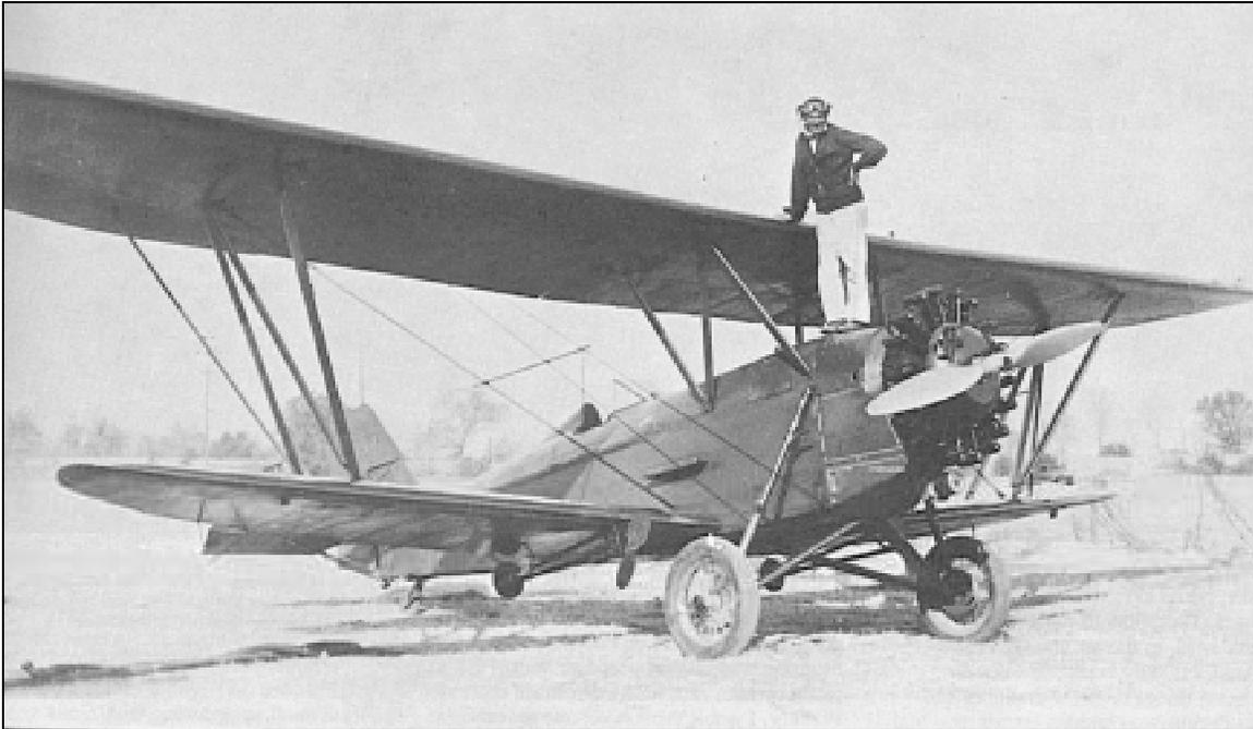
Independent Crop Dusters New Standard D-25 sprayer powered by a Wright J-5 225 hp air-cooled radial engine. Pilot Brown is standing on upper engine cowling, which is where the aircraft is fueled. Photo courtesy George Sanders from “Low & Slow,” by Mabry Anderson.
