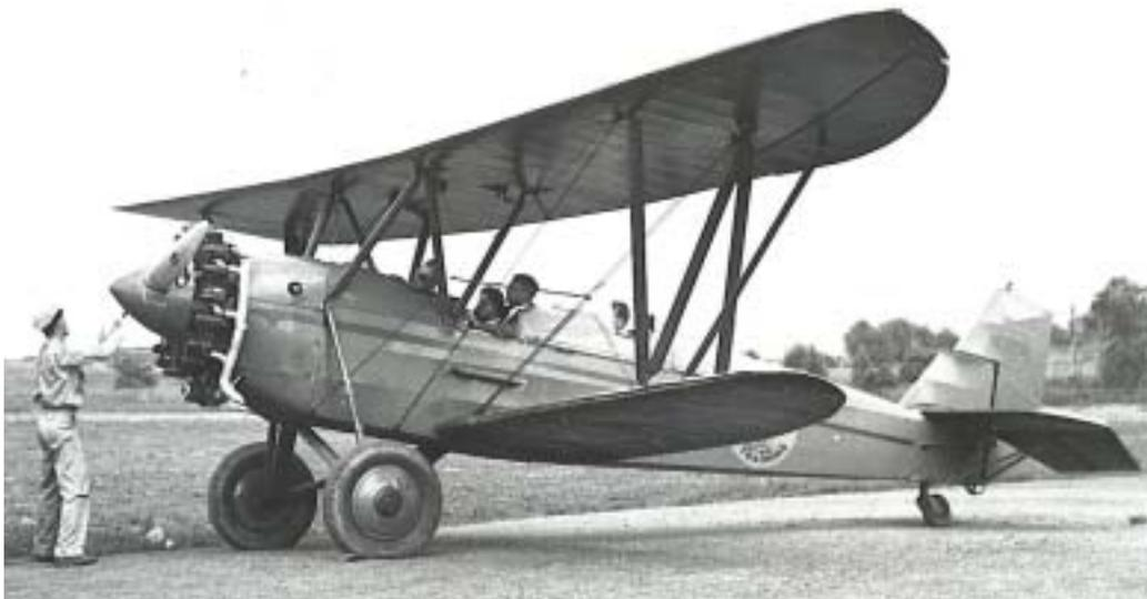
Above, NC9756 serial 105, originally a model D-24 now converted to a model D-25 by factory by installation of the Wright J-5, 225 hp engine. Also installed were mechanical brakes and a pneumatic tail wheel to replace original tailskid. Photo from Peter Bowers.
