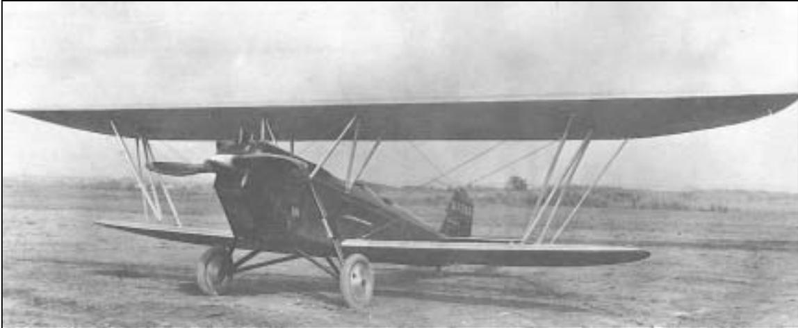
Above, the Gates-Day GD-24 prototype, NX7286, serial number 101. Power was a 180 hp Wright "Hisso" water-cooled motor.
