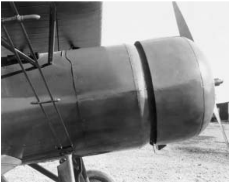
Above, NACA official photograph of the Curtiss AT-6, left unmodified with engine exposed and right with Fred Weick's pressure cowling.
