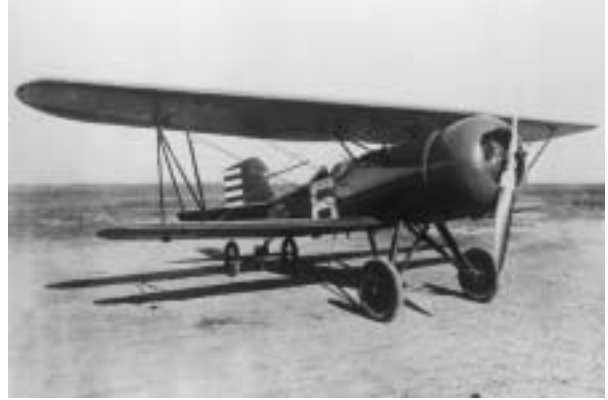
Above, NACA official photograph of the Curtiss AT-6, left unmodified with engine exposed and right with Fred Weick's pressure cowling.
