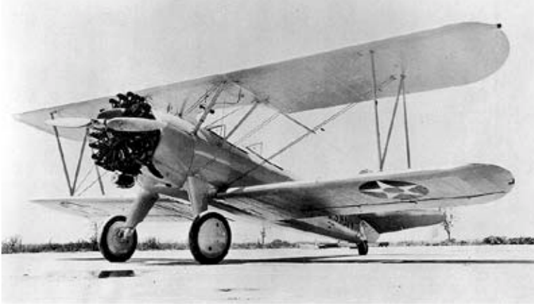
Left, a Model 73/U. S. Navy NS-1 (1934-1935) manufactured by the Stearman Division of Boeing Airplane Company. Markings are for Army Air Corps.
